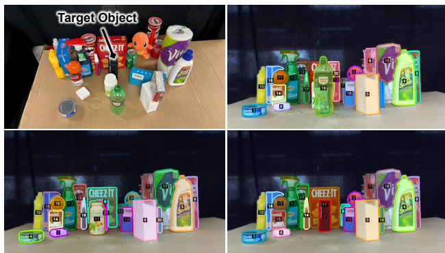
Fig. 1. (Top Left) Bird’s eye view of an experiment. (Top Right, Bottom Left/Right) Segmented images from the robot’s view before a pick until the hidden black box (target) is retrieved. The target is labeled 0 when found.
